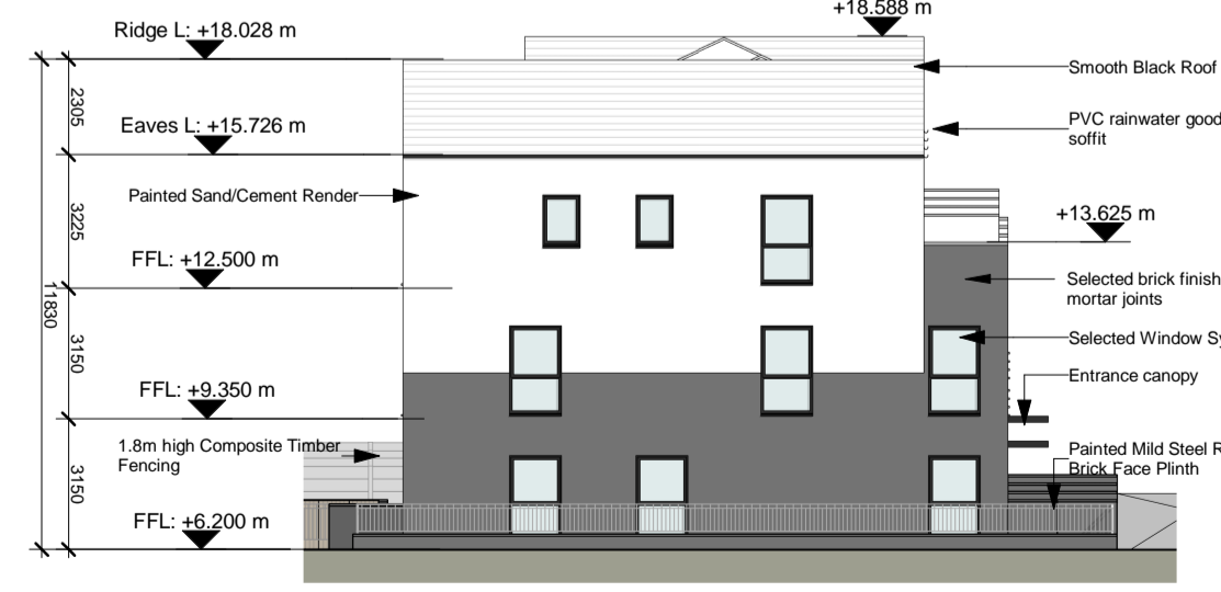
7 Duplex Block K North Elevation 1 : 200
